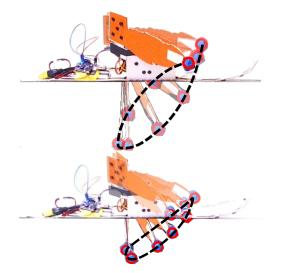
Fig. 13: Top: the gait produced by the right fin after iteration 10 with fin A. Bottom: the gait produced by the right fin of the robot after iteration 3.
