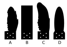
Fig. 7: The four different design of fins used for the presented robotic device. Designs A and C are accurate reproductions of the actual shape of sea turtle fins, namely *Caretta caretta* (A) and *Natator depressus* (C). Designs B and D are simple rectangular and ellipsoid shapes.
