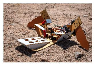
Fig. 1: A robot made from a multi-layer composite learns how to move across sand in the Arizona desert.
