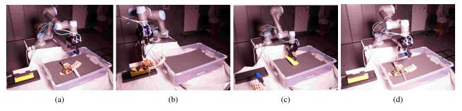
Fig. 6: Sequence of actions the robotic arm executes in each learning cycle: (a) First the robot under test is located in the testbed, grasped and then (b) subsequently moved into a resting position. The robotic arm proceeds to (c) smooth the testbed with a tool. Finally, the robot under test is (d) put into its initial position and the next trajectory is executed.
