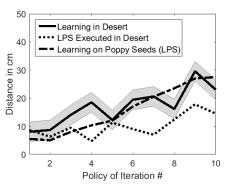
(b) Comparison between policies learned for fin design A. The algorithm was initialized with the same random number generator for learning. Due to a technical issue only pixel distances were recorded for learning in the desert. For comparability those pixel distances were transformed into centimeters but are attached with a variance of about 3.5cm.
