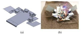
Fig. 5: The initial "flat body" design of the robot. The front of the robot buried into the sand during motion. The body was later curved
