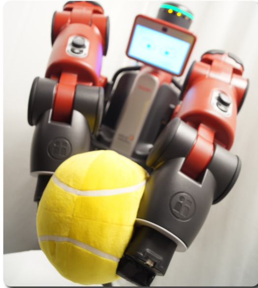
Fig. 1: A bimanual robot learns to lift an object while simultaneously identifying synergies among the control variables.
